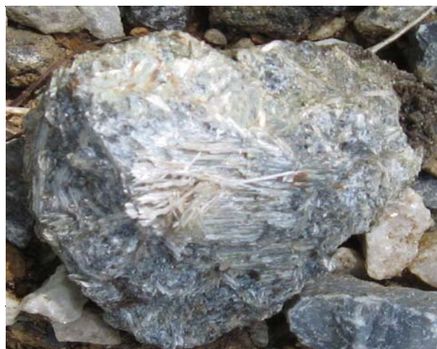
Example of naturally occurring asbestos ore found on the site
