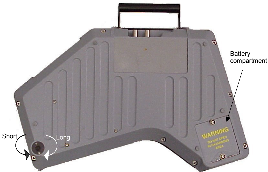
Figure 4-3. Location of Pathlength Adjustment and Battery Compartment
