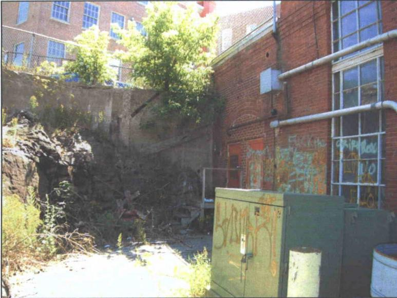
4. Thurs. 7/14/11: Rear, north side, of the substation showing the doors into the 4000-gallon #2-oil AST and a vent pipe on the side of the building above the door [see Photo-6 below].
