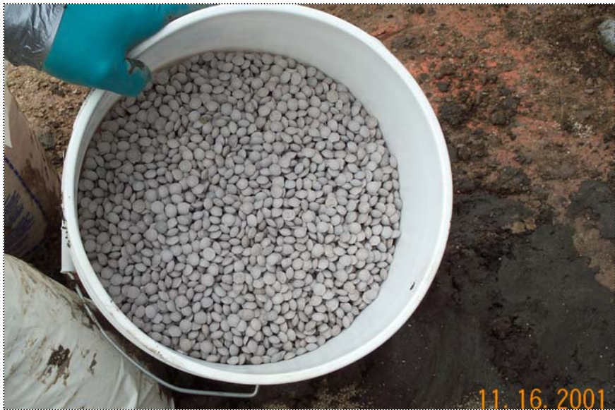
DCP1286 - View of the bentonite tablets for well SS-12
