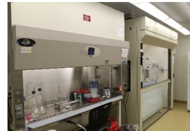
Certified Biosafety Cabinet and Chemical Fume Hood that houses a Janus Automated Workstation for high throughput sample processing.
