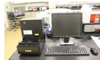
ECL machine capable of detecting biological toxins and proteins.
