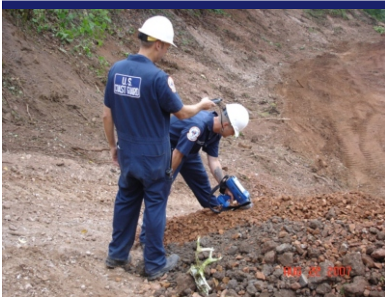
Photo 1 XRF testing of mercury in tailings removed from Main Tailings Pile - West slope.
