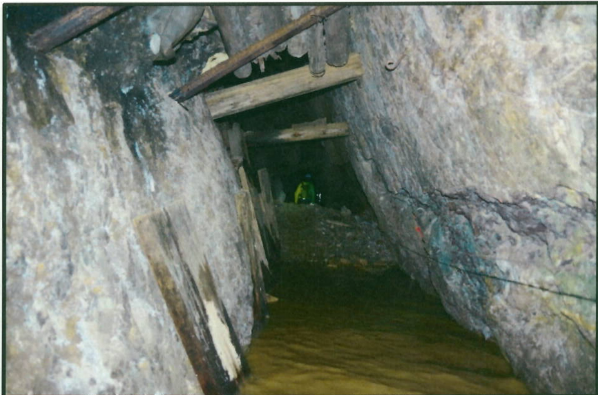
Photo 42: Debris pile at 44 Raise 36+82 looking outby; Note water ponded behind pile
