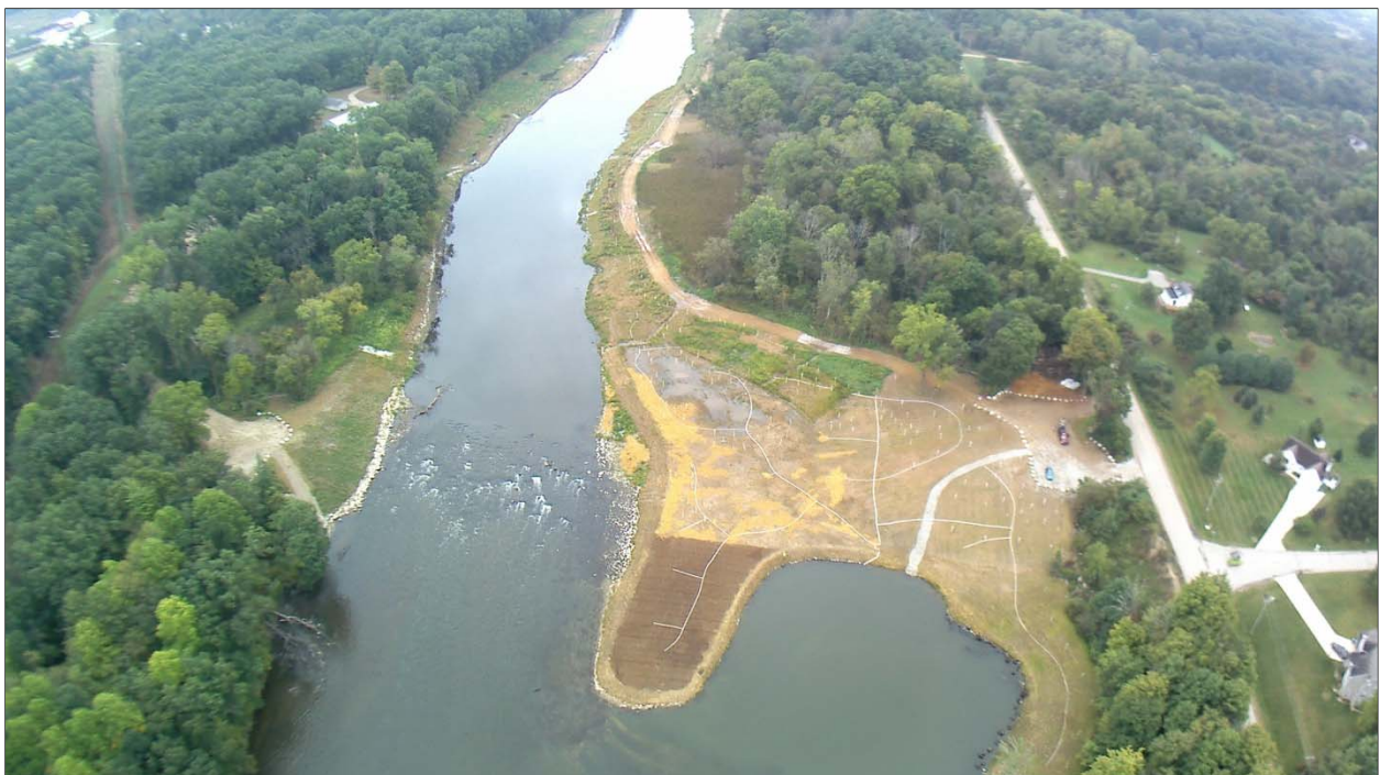
Photo 56: View after removal of former WCS and restoration of former WCS corridor and plunge pool area, looking upstream.
