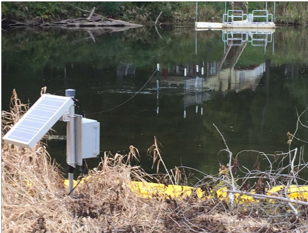
Photo 2: Turbidity monitor set up downstream of work area (2016).
