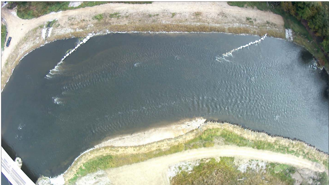
Photo 20: Aerial view of J-hooks installed on BRSA 3 bank (October 2017).
