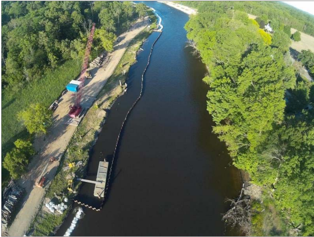
Photo 23: Aerial view of BRSA 4 sheet pile cofferdam (June 2017).
