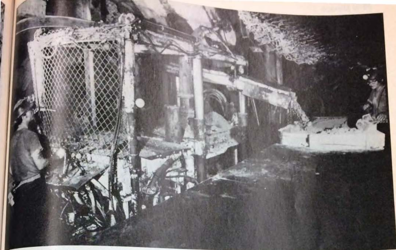
Calweld blindhole raise borer develops 54-in.-dia holes while automatically sending muck to cars.
