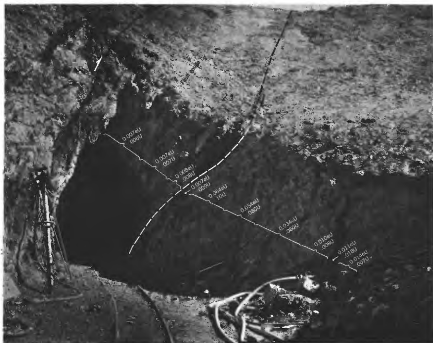
FIGURE 16.—Adit in gouge zone of thrust fault, NW \frac{1}{4} NW \frac{1}{4} sec. 9, T. 28 N., R. 92 W. Percent equivalent uranium (eU) and uranium (U) shown for chipped samples collected along zone indicated by bracketed line.
