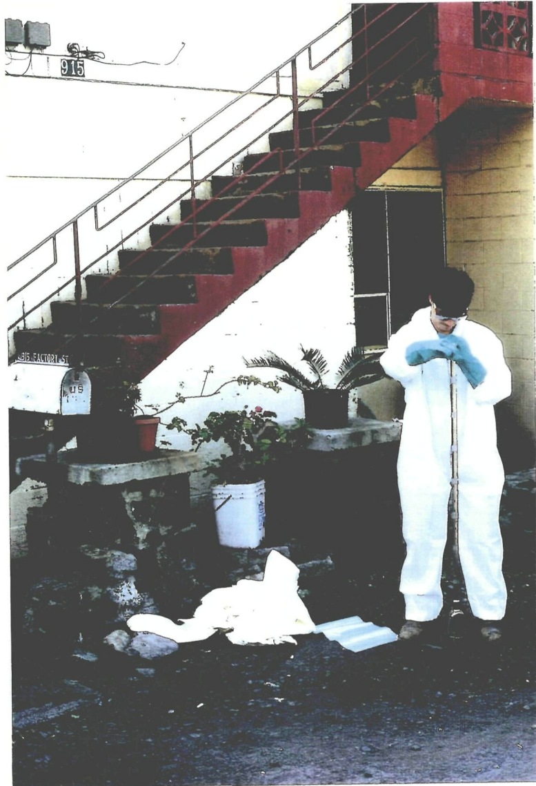
Photo 1: TAT collecting soil sample with hand auger at 915 Factory Street
