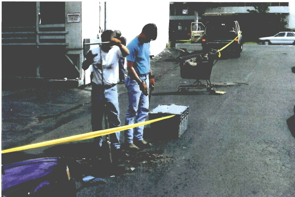
Photo 4: The TAT collecting soil samples beneath the asphalt in the center of Factory Street
