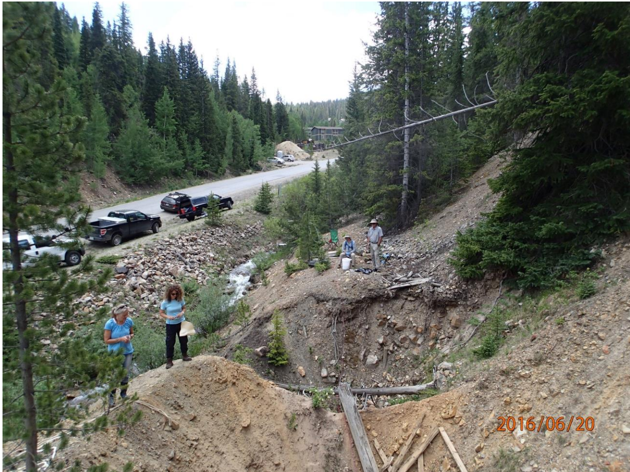
Figure 9: Photograph showing the Collapsed Two-Compartment Puzzle Extension Shaft, the Pumping and Dye Mixing Station Established at the Shaft Collar, and the Close Proximity of the Creek to the Shaft.
