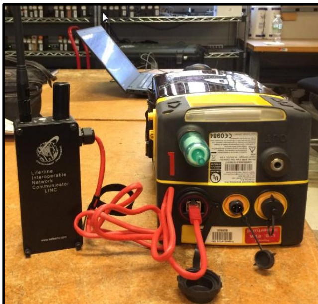
Complete SPM Flex Setup (LINC, RJ45 cable and Instrument)
