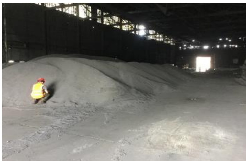
Figure 3: "Green coke" waste piles are one of several primary sources containing high levels of carcinogenic PAHs migrating from the facility parcel through the stormwater system and found at elevated concentrations in settling ponds.
