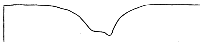
FIG. 9.—Diagram to illustrate the widening of a valley flat by erosion. (After Chamberlin and Salisbury.)
