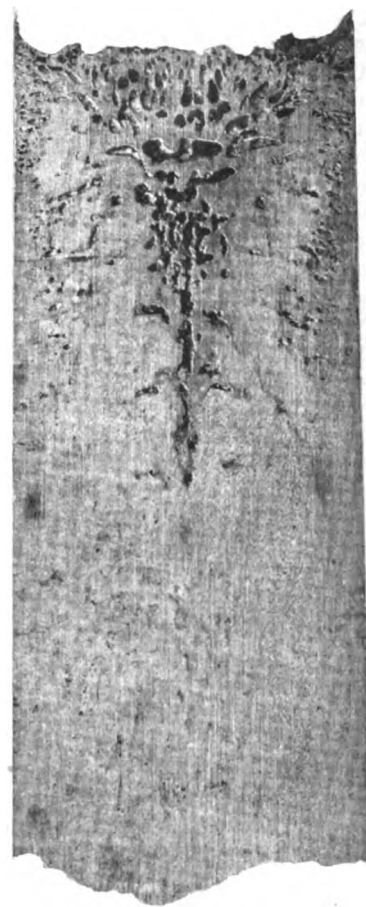
Hammered Steel Ingot, Showing How the Gas Bubbles Cause Little Volcanoes to Erupt Liquid Steel Until the Crust is Solidified.
