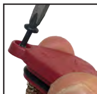
FIGURE 36 INSTALL CAPTIVE SCREW
