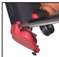
FIGURE 34 REMOVE HINGE SCREW
