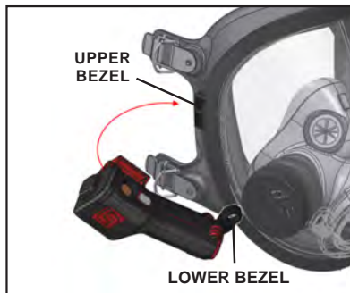
FIGURE 17 ROTATE TIC OVER UPPER BEZEL
