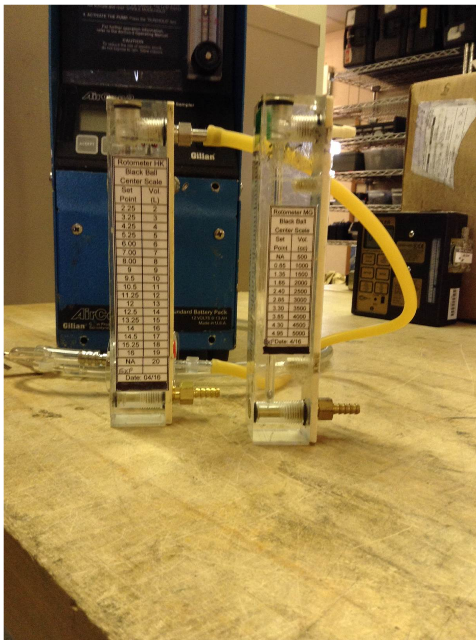
FIGURE 3. Rotameter Flow Rate versus Set Point
