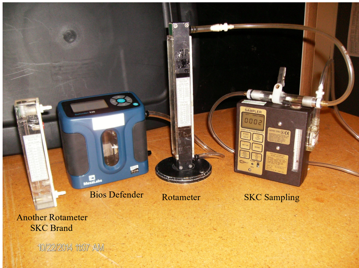
FIGURE 3. Field Calibration of a Rotameter
