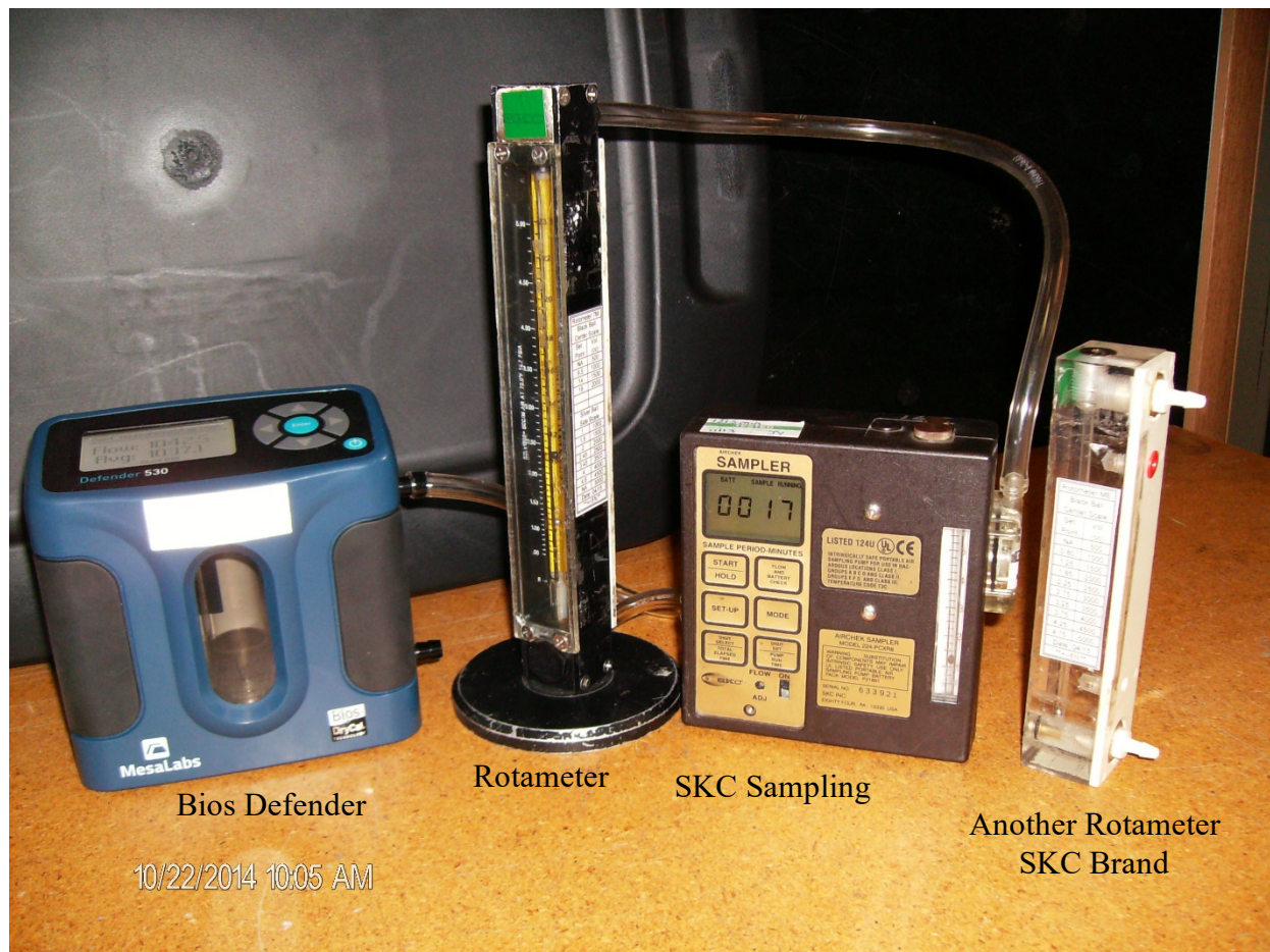
FIGURE 1. Calibration Train for Calibrating Rotameters
