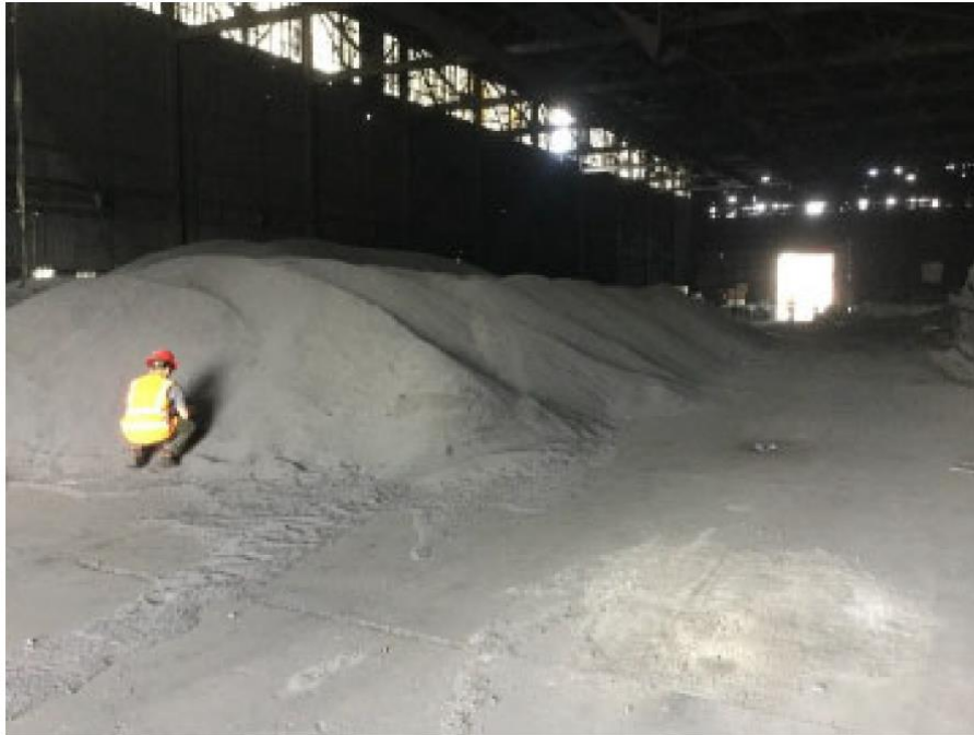
25 "Green coke" waste piles containing high levels of carcinogenic PAHs. One example 26 of uncontrolled waste material.
