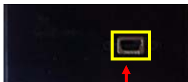
5V USB charging port on the bottom of the Gen 3 LINC
