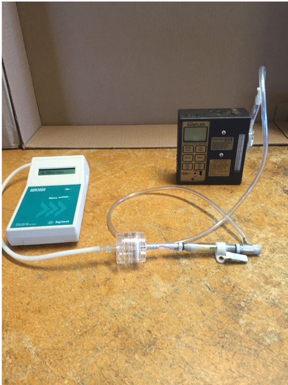
FIGURE 2. Calibration Train with Personal Sampling Pump and Filter
