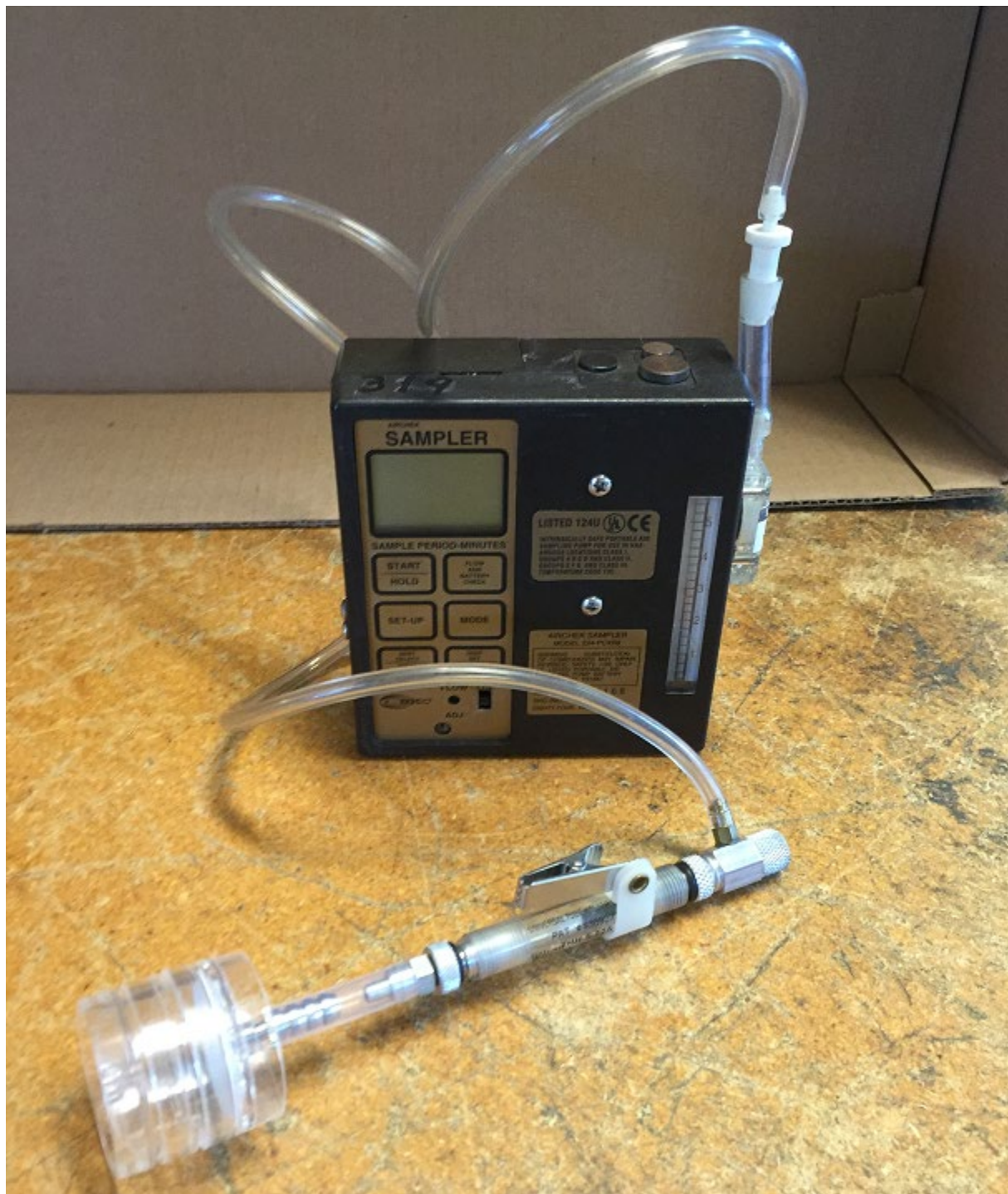
FIGURE 5. Sampling Train for an Area Sampling Pump
