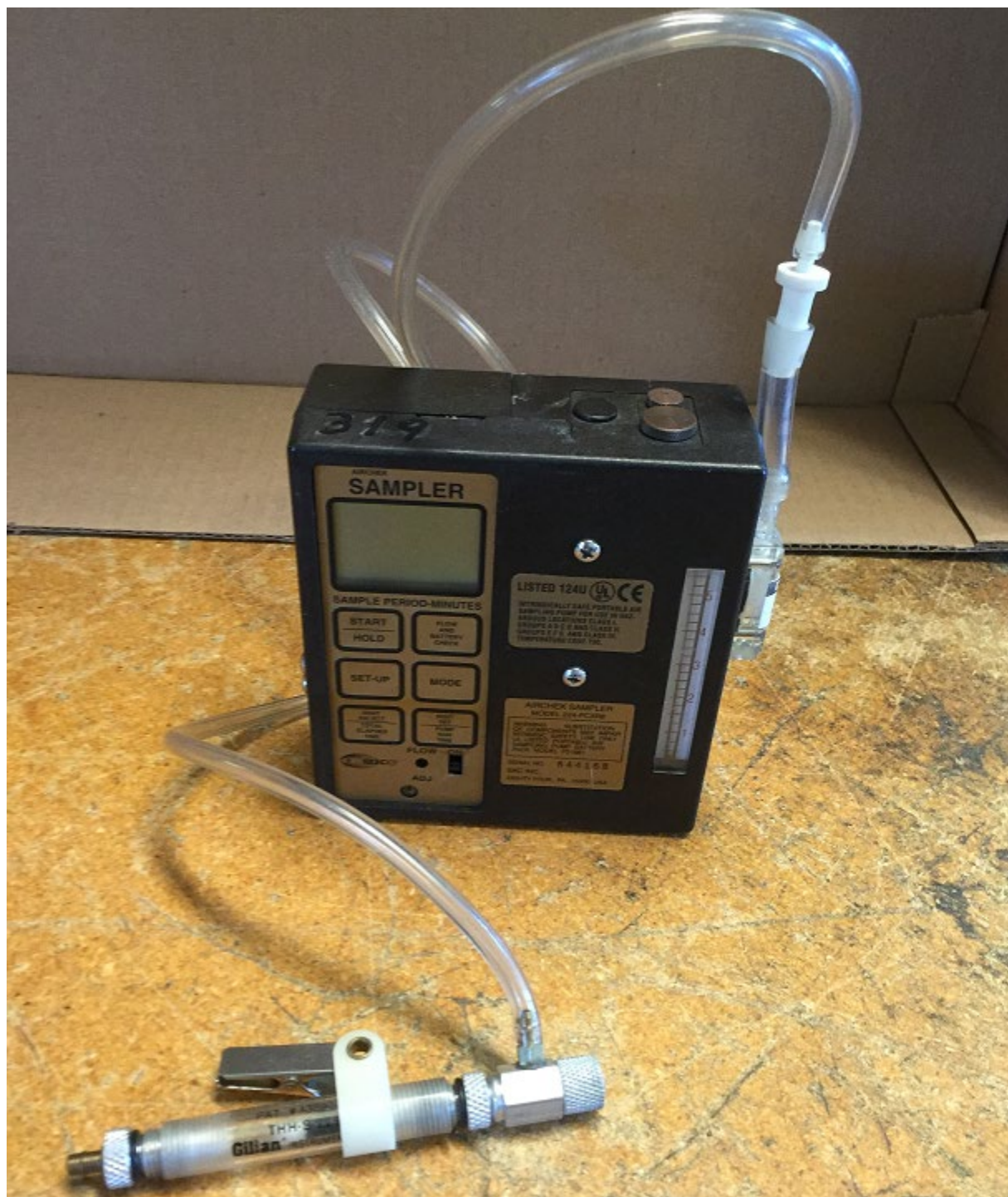
FIGURE 4. Sampling Train with Personal Sampling Pump
