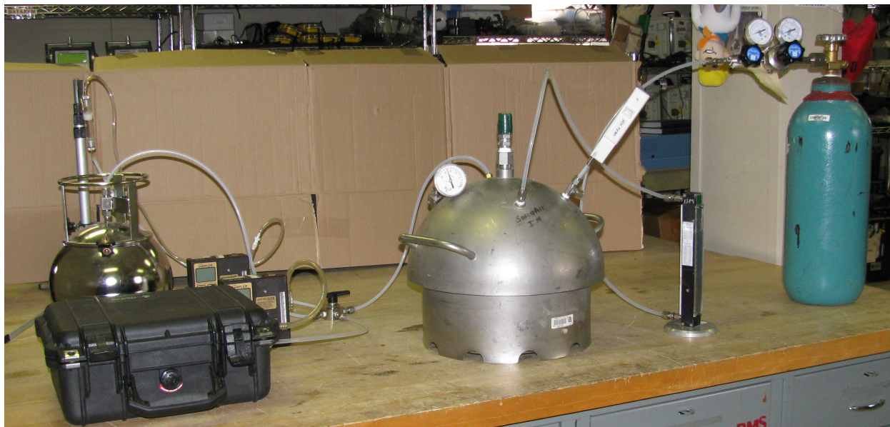
FIGURE 1. Picture of Flux Chamber Sampling Train
