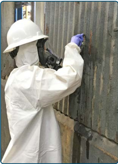
A worker samples the inside wall of Building 57 for contaminants.
