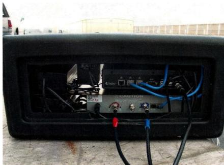
8. Connect the control cable to the cam connection on the back of the modem in the PSU-CU.
