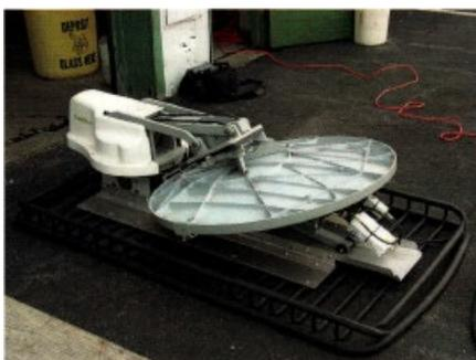
3. If the dish is properly stowed, the dish icon with an arrow pointing down to represent the stowed position is displayed.
