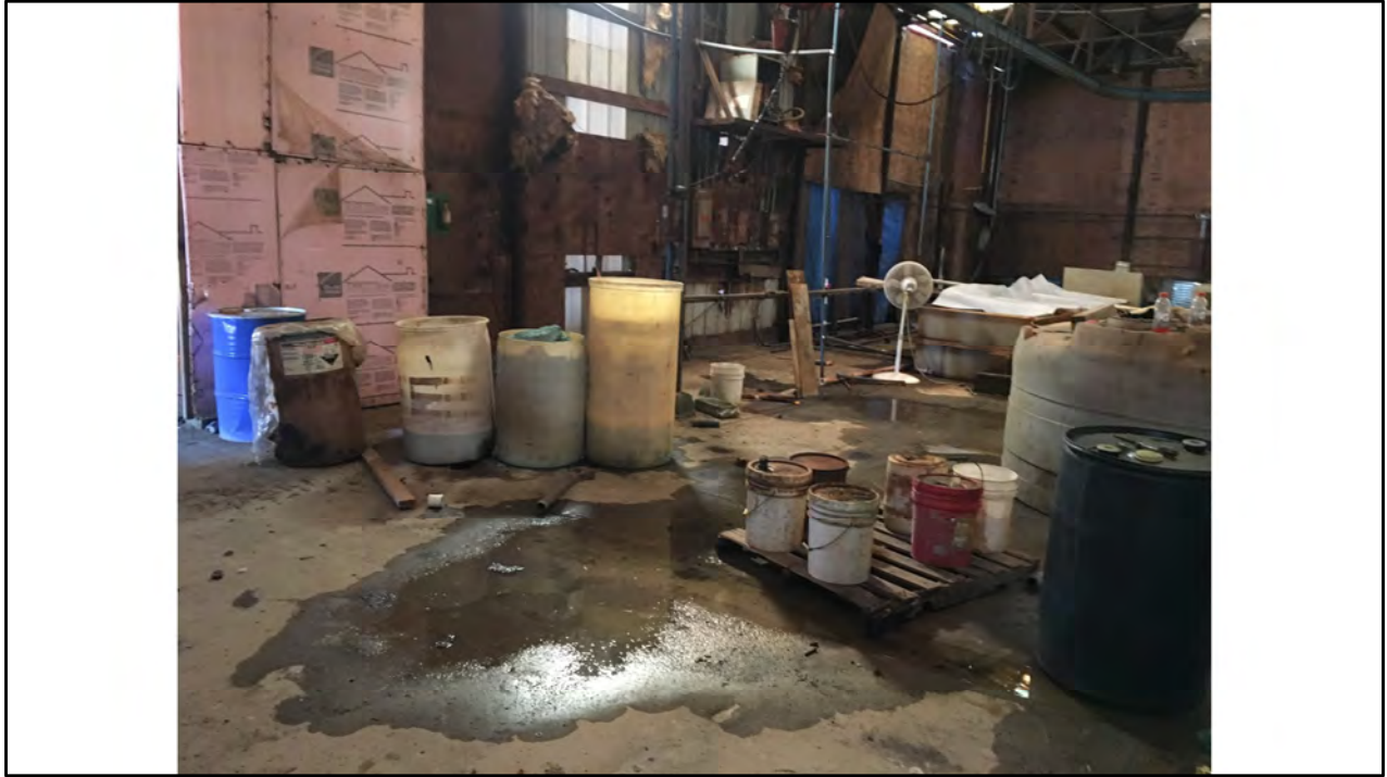
CCS, 10/5/2020, CEI AI# 3106, Livermore Industrial Plating: Site photo. The facility claims product status for all material. Floor is designed to drain to a sump then WWT operation. Sump and associated trenches are filled with liquid (reported to be rain water). Liquid stands on floor.
