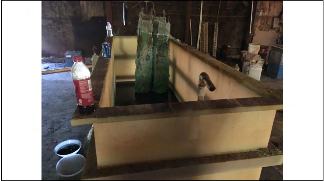
CCS, 10/5/2020, CEI AI# 3106, Livermore Industrial Plating: Site photo. The facility claims product status for all material in dip tank. This is nickel plating solution.
