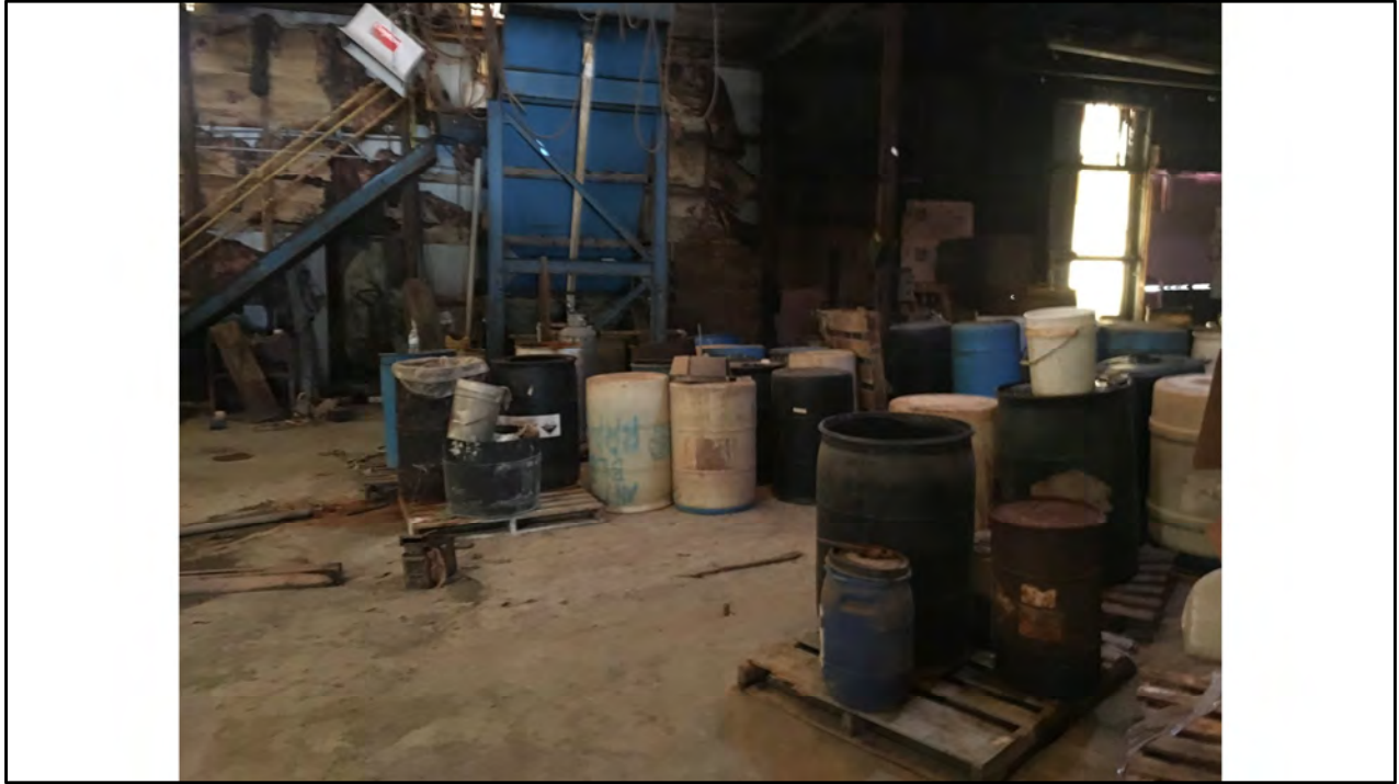
CCS, 10/5/2020, CEI AI# 3106, Livermore Industrial Plating: Site photo. The facility claims product status for all material. Floor is designed to drain to a sump then WWT operation. Sump and associated trenches are filled with liquid (reported to be rain water). Liquid stands on floor. The upside down containers are empty.
