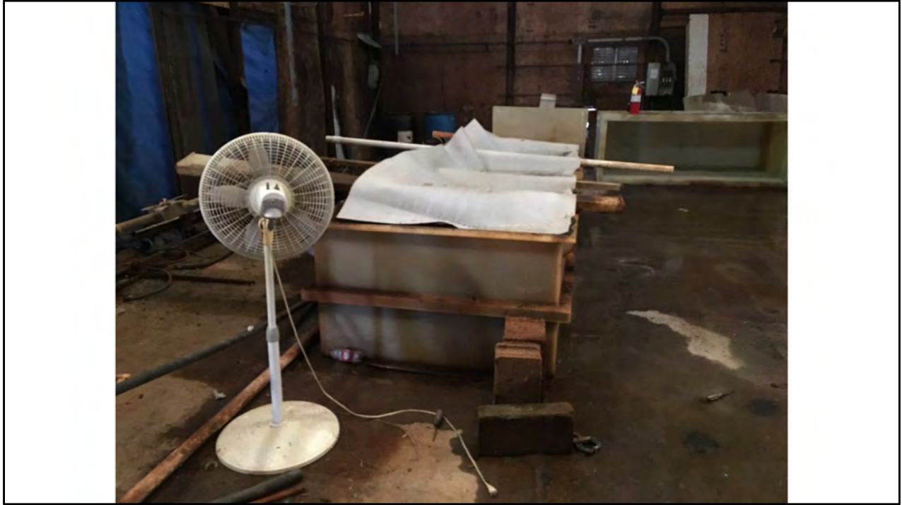
CCS, 10/5/2020, CEI AI# 3106, Livermore Industrial Plating: Site photo. The facility claims product status for all material. Floor is designed to drain to a sump then WWT operation. Sump and associated trenches are filled with liquid (reported to be rain water). Liquid stands on floor. This dip tank is about to run over. It is staged under a leaking roof. Zinc plating solution
