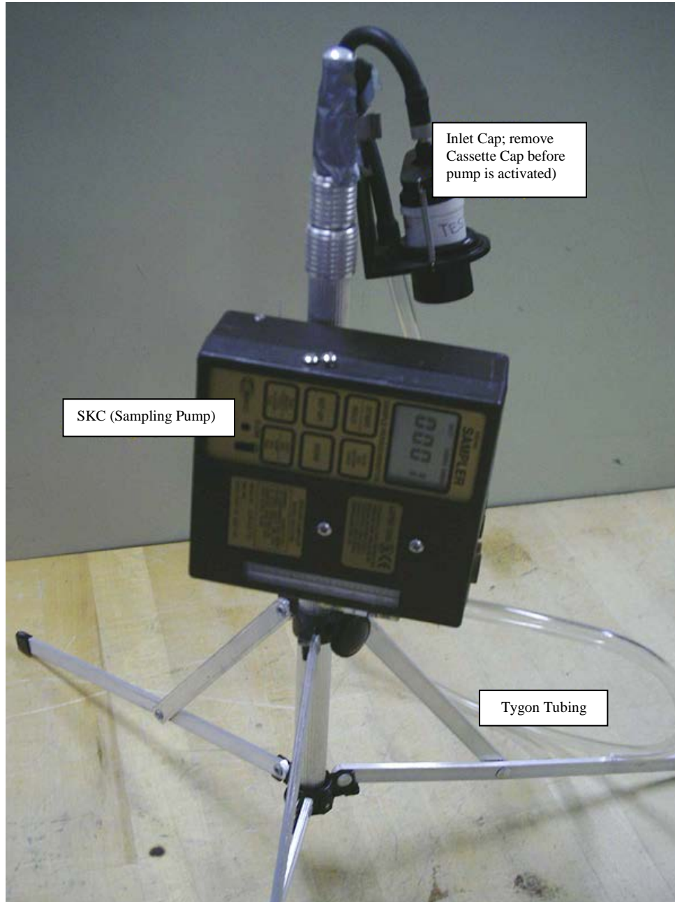
FIGURE 5. Personal Sampling Train for Asbestos
