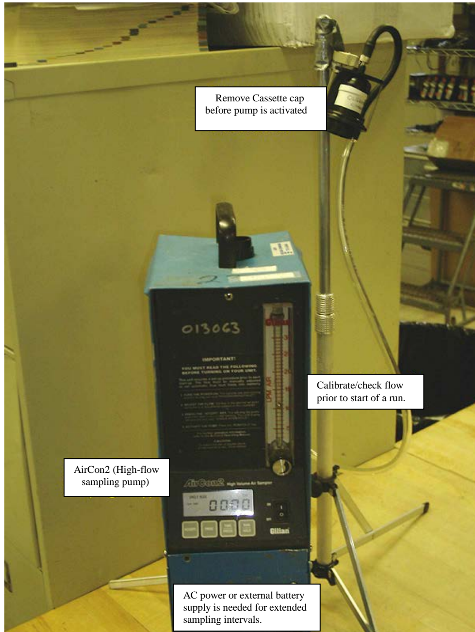
FIGURE 6. High Flow Stationary Sampling Train for Asbestos
