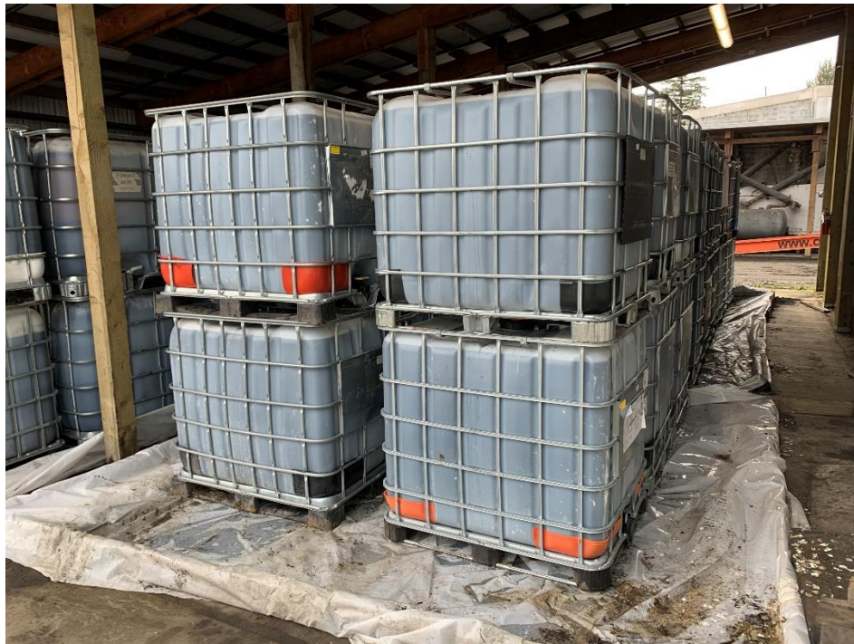
Figure 3: Totes containing an estimated 24,000 gallons of waste located under the Lean-To with no security or secondary containment.
