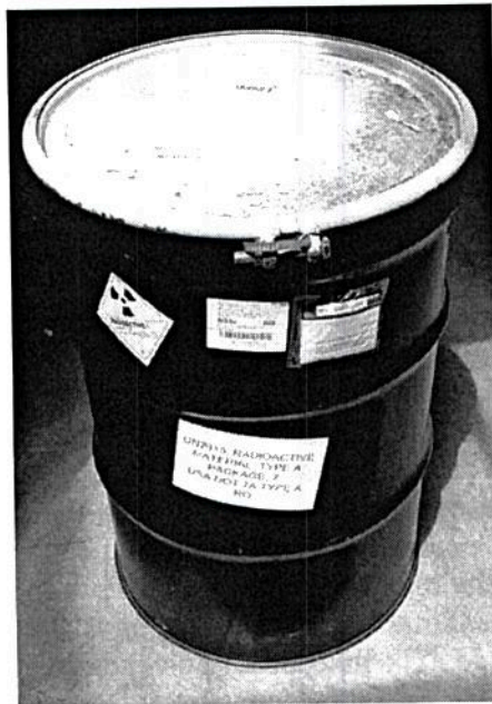
Figure 1: 55 Gallon Overpack with Ubeds as Received
