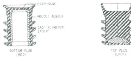
Figure 3.11: Schematics of the plugs involved in the two plug system. Note the color difference between the plugs. The color makes identification easier when drilling out a problem well where the cement has set p in the pipe.
