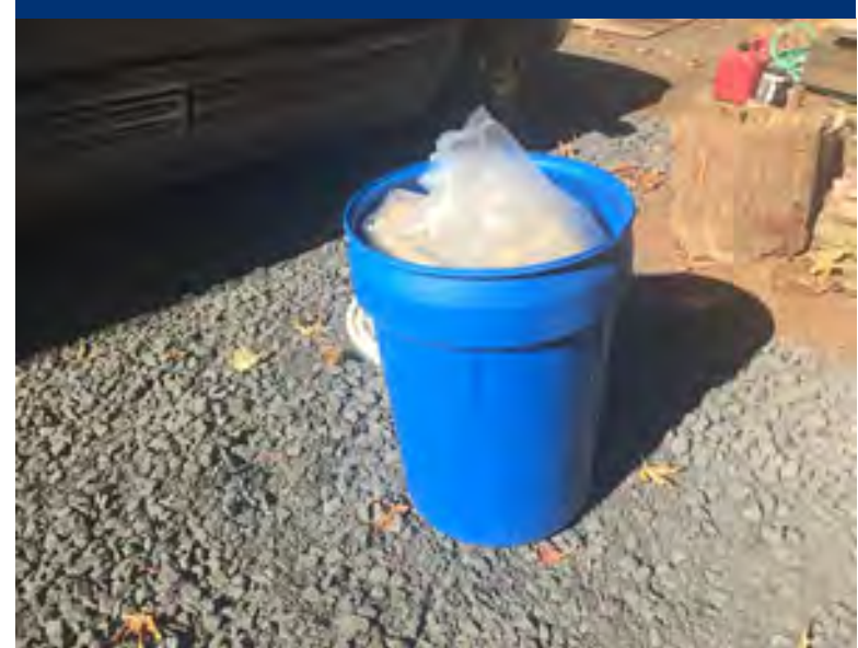
Photo 35 Mercury flasks placed in overpack container, with sorbent.
