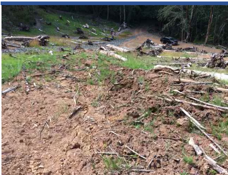
Photo 51 Looking downslope at right bank slope failure of Adit Creek seep at BS01.
