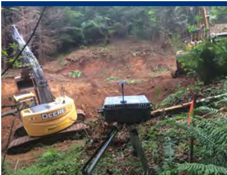
Photo 3 Air monitoring for dust particulates with DustTrak at STA 5+50 LB.
