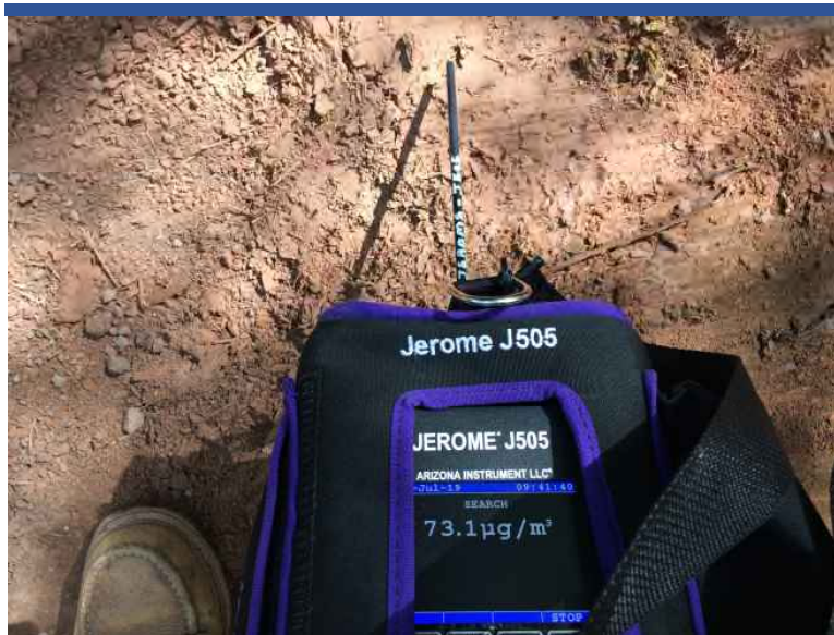
Photo 21 START conducting mercury vapor monitoring of exposed lens of ashy material in OPWA Lower/North unit.
