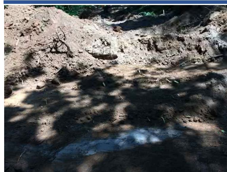
Photo 20 Exposed contaminated lens of ashy material in SE extent of OPWA Lower/North unit.
