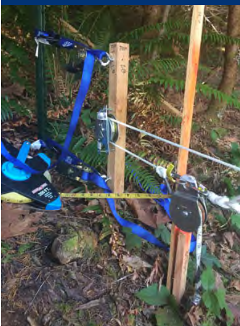
Photo 22 Stream profile measurement system detail.
