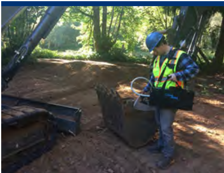
Photo 16 START scanning bucket of excavator for mercury vapors with Lumex.
