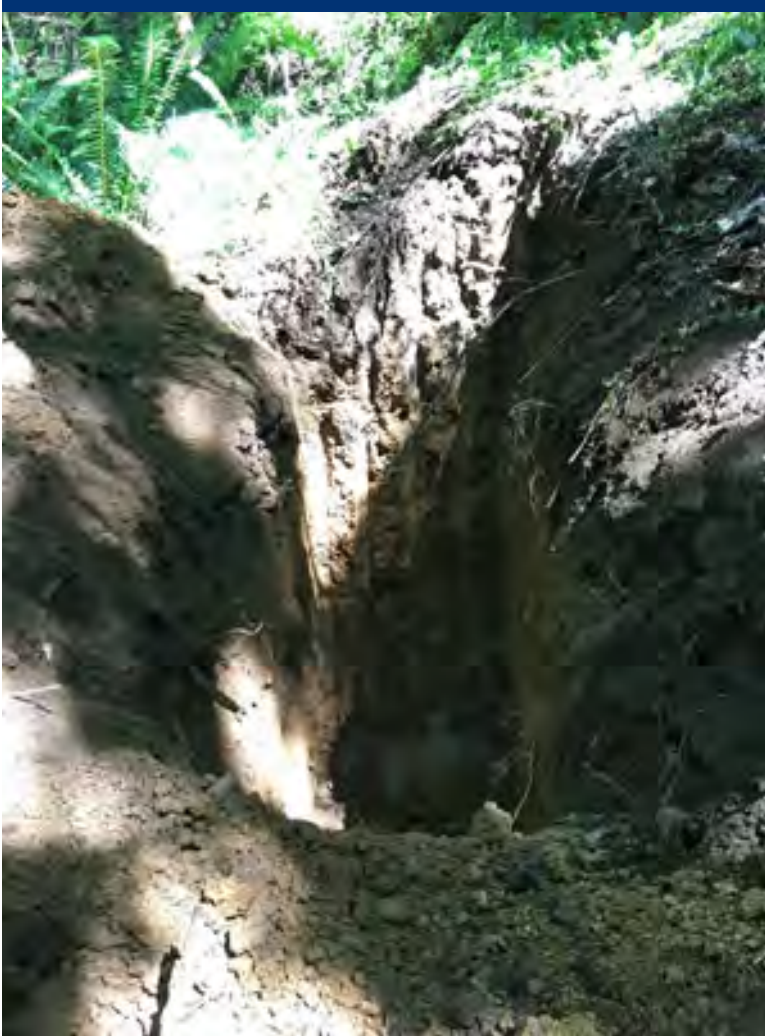
Photo 7 Borrow Source test pit sampling activities.
