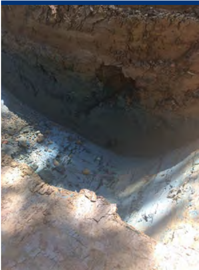
Photo 5 Test pit placed at STA 6+25, along left bank trench floor, revealing clay cap cover at 5 feet-plus deep.
