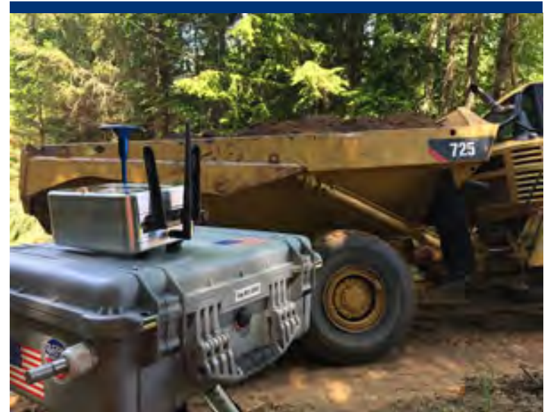
Photo 2 Vaporized dust monitoring station near Furnace Creek removal activities.
