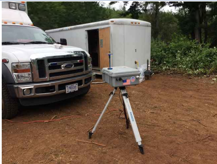
Photo 1 Air monitoring station AS-CP Dusttrak, COMMs rig, and START equipment trailer.
