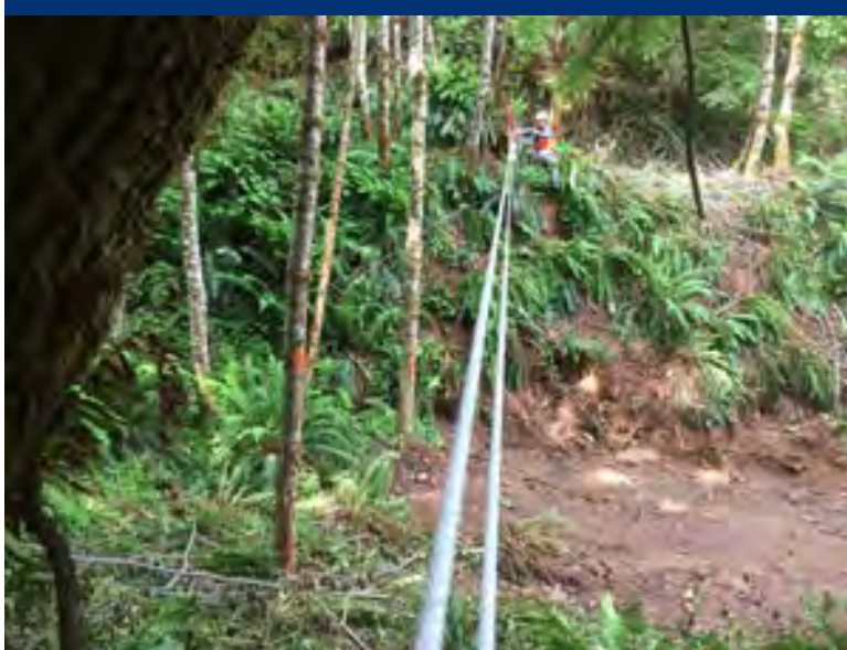
Photo 24 Stream profile measurement system at Station 0+00.
