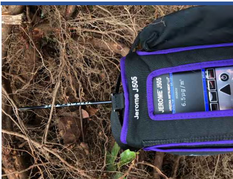
Photo 7 START conducting mercury vapor monitoring of stockpiled root wads with Jerome J505.
