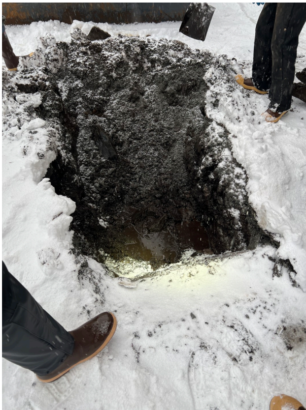
Overview of ground water at 15" below the surface.
