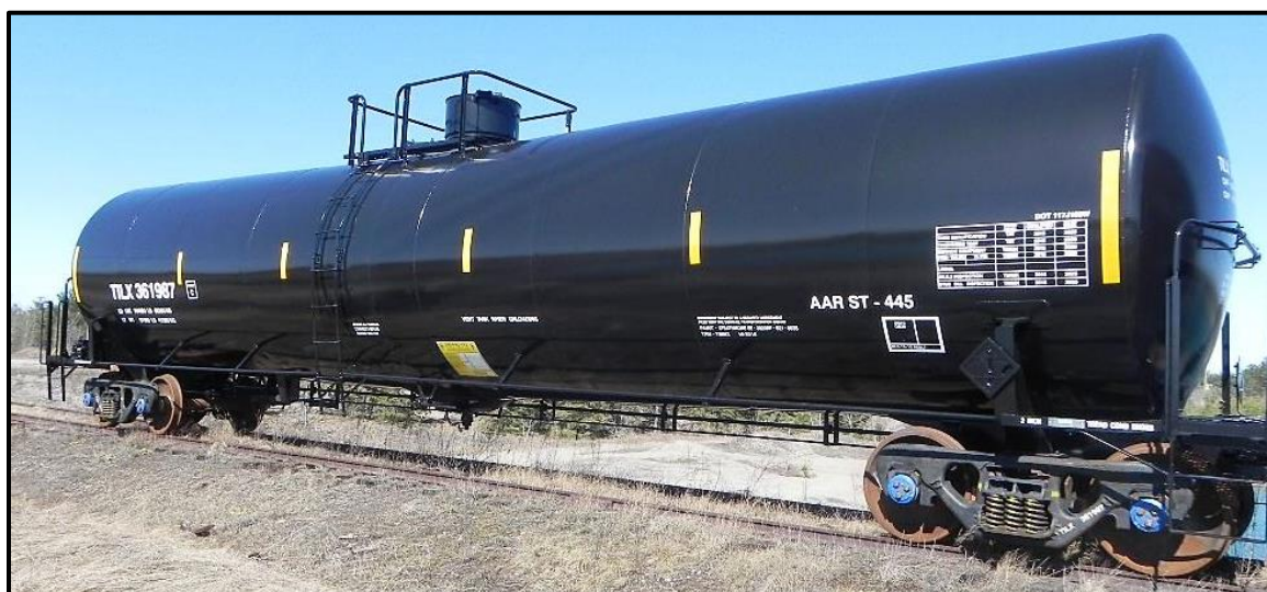
DOT/TC-117J100W Tank Car for Flammable Liquid Service
