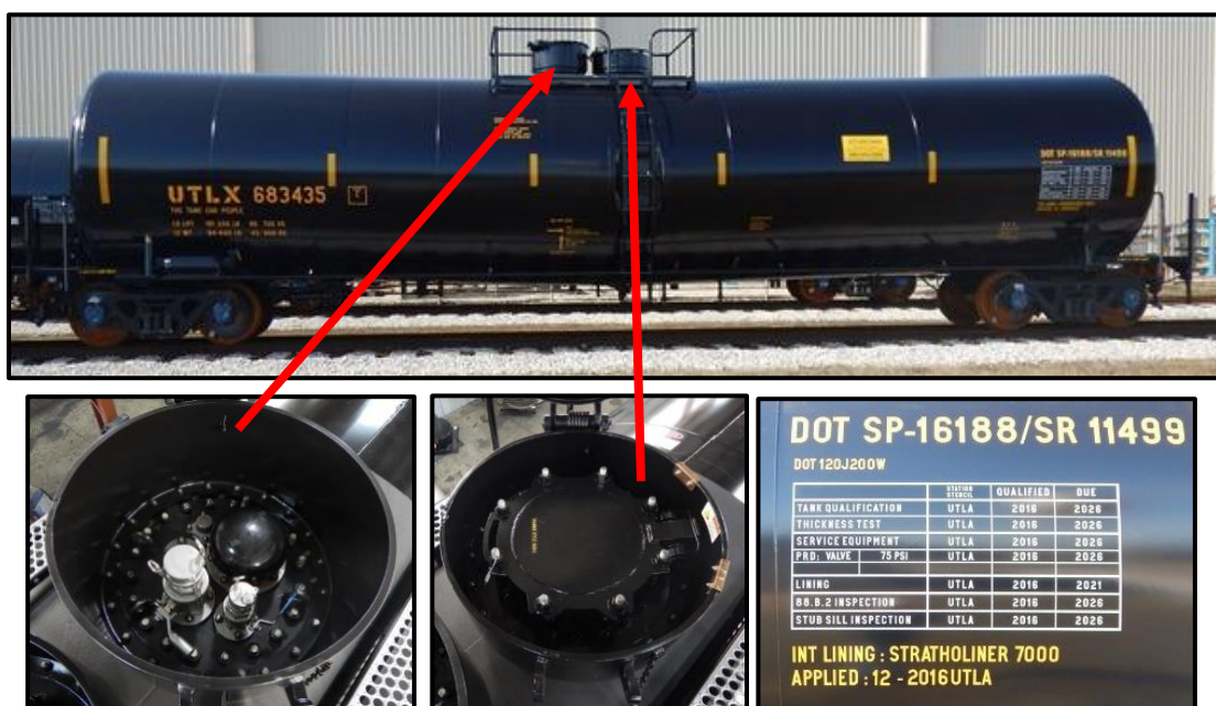
DOT-120 Tank Car for Flammable Liquid Service. Note the protective housings.
