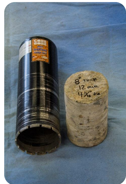
Concrete Coring Bit 8" Concrete Foundation Core 12 minutes to Cut
