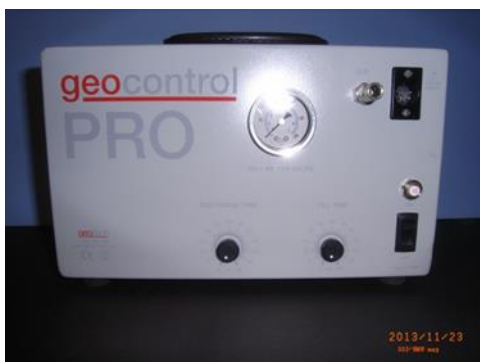
Air Activated Bladder Pump
