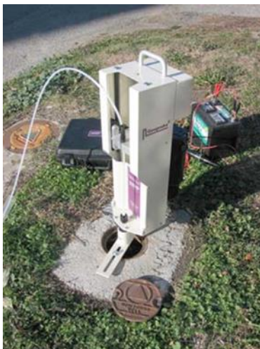
Mechanical Bladder Pump
