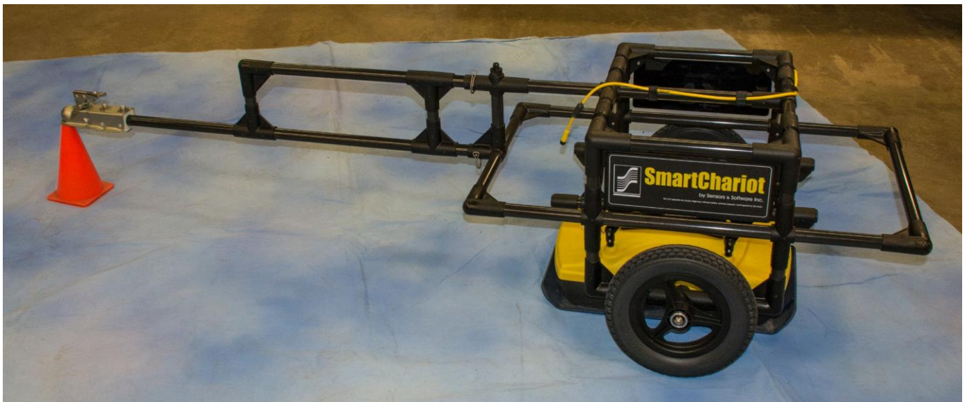
GPR configured to be towed by ATV for large sites.
