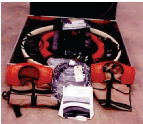
EM34: Orange and white round antennas in shipping case. Options for cables, 10M, 20M and 40M in length allow for shallow and deeper exploration.
