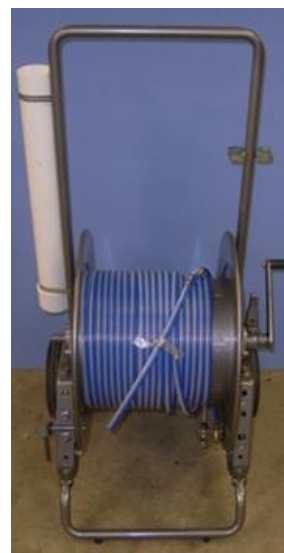
Air – Water Lines for Bladder Pump
