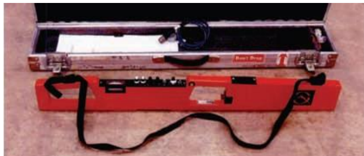
EM38: Instrument has one-meter coil spacing for near surface investigations.
