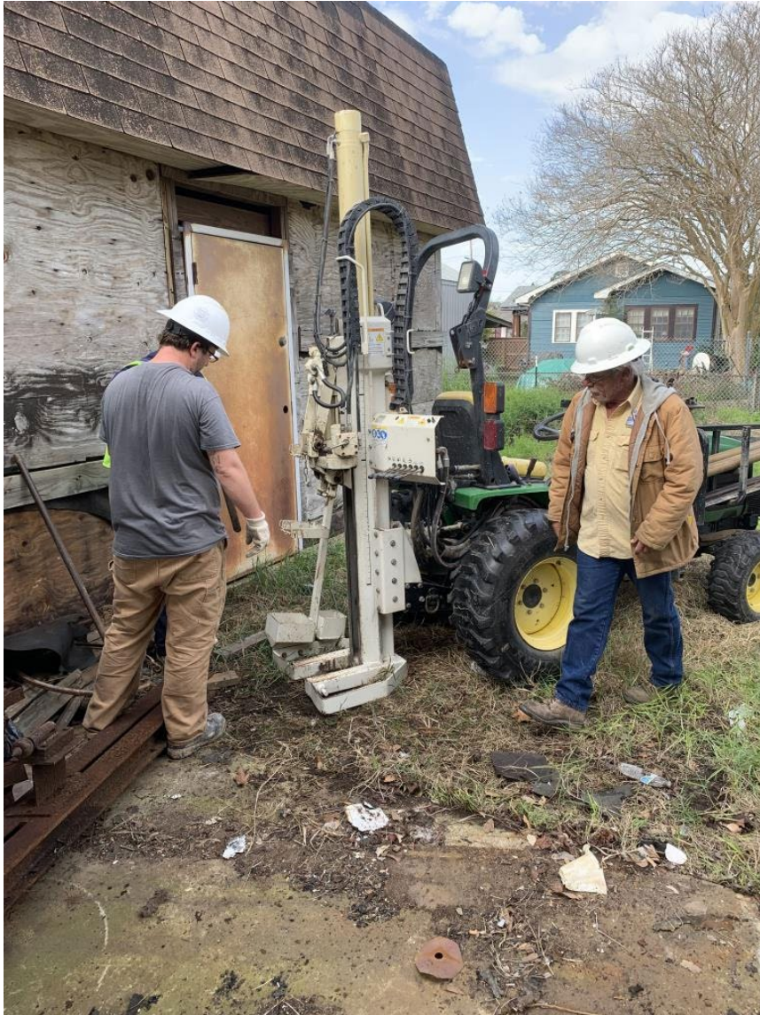
Soil sample being extracted next to the secondary building
