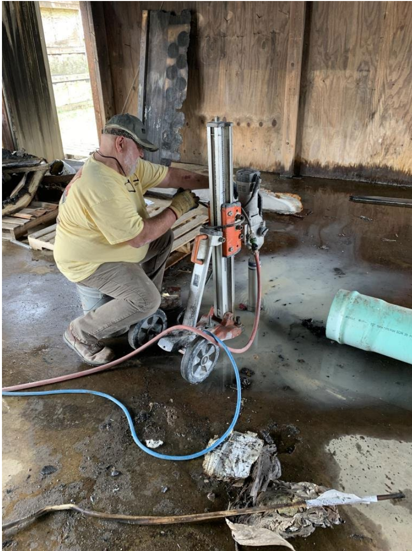
Core concrete sample being extracted from the floor slab
