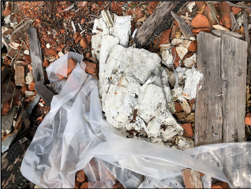
March 2022 – Air-cell pipe insulation confirmed to have 30% chrysotile asbestos
