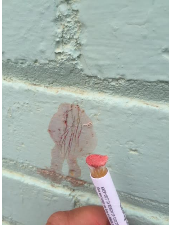
Photo 5. Positive lead check on the green paint on the north wall of the hotel/lounge building.
