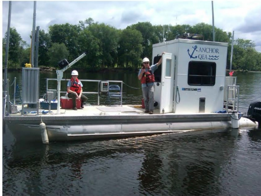
AQ-1 24-foot Pontoon Coring Boat with hard cabin and twin engines
