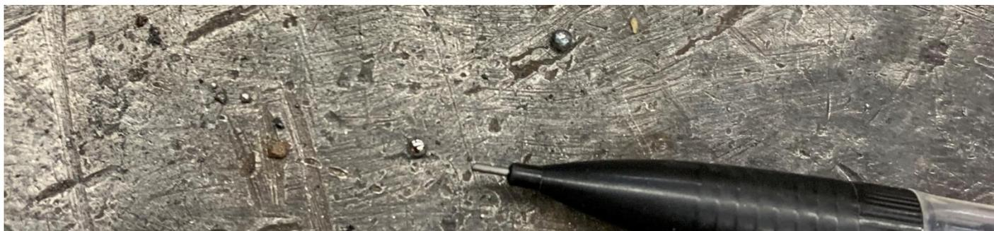
**Photo Description:** Elemental Mercury (where the pencil is pointing) in addition to welding beads, located in the Welding Shop.
