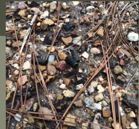
M6 Propellant on the Ground
