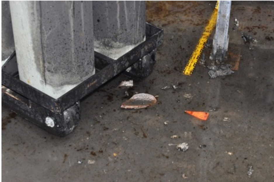
The fractured section of the Y-strainer was Recovered in a walkway near reactor K-8 and West of the Y-strainer.
