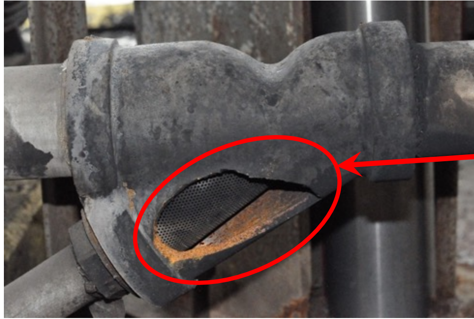
The failed Y-strainer
