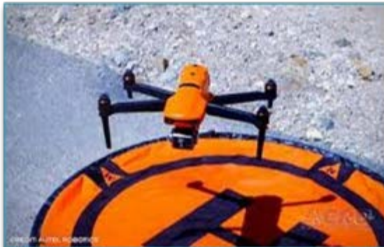
TCEQ's new Autel EVO II Dual Drone w/thermal imaging and 8x Optical Zoom
