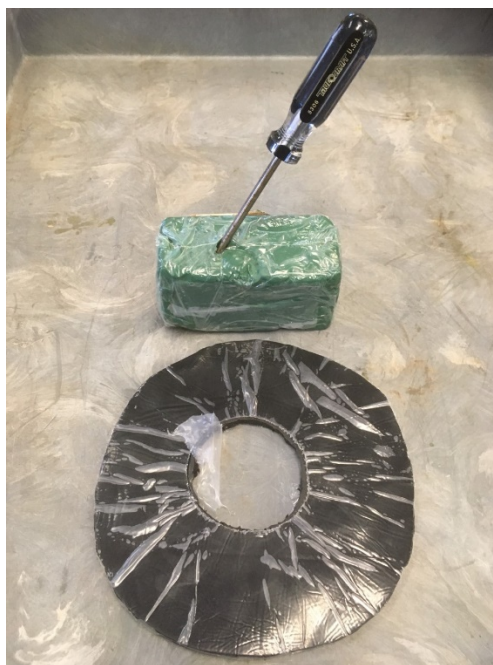
Figure 6. A compressible gasket or clay may be used as sealing material.
