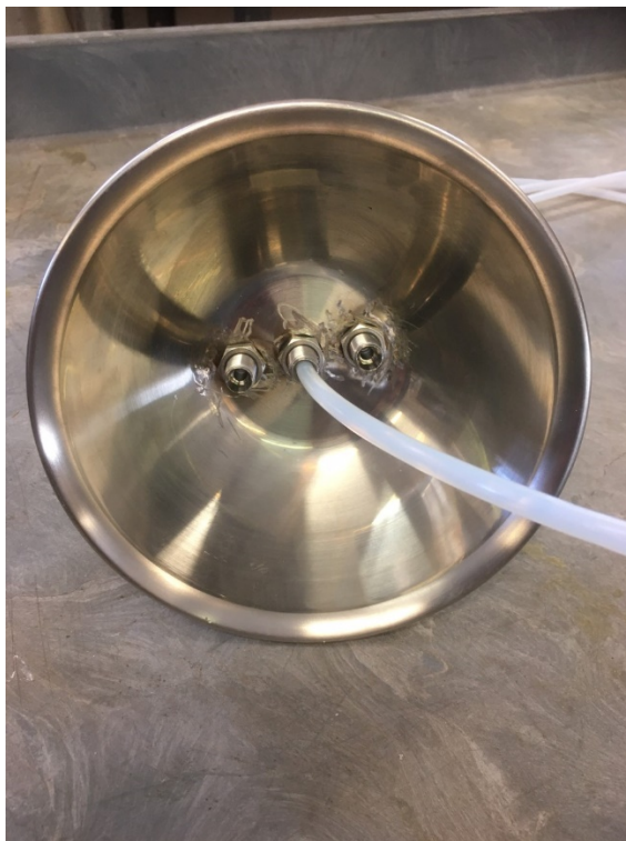
Figure 4. Tubing which connects sub-slab soil gas probe to sample bag in vacuum box.
