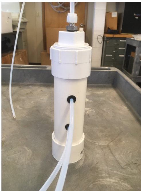
Figure 5. PVC pipe with grommets as shroud.
