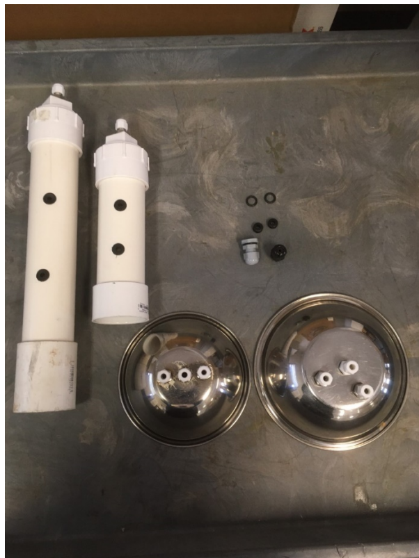
Figure 3. PVC pipes, bowls, and fittings for use as shroud.
