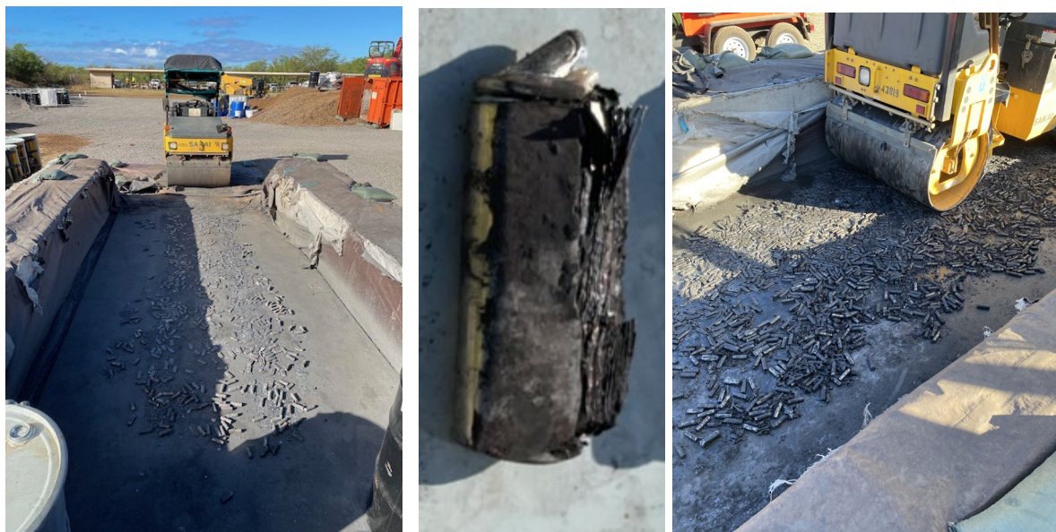
Figure 14: Using a drum roller to crush cylindrical batteries (left and right) and get to a final product for disposal (center).
