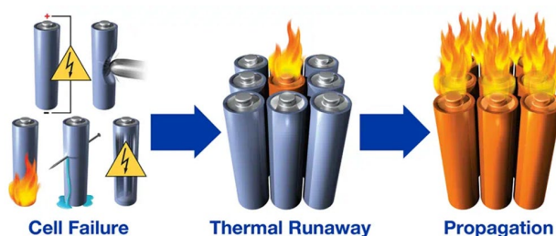
Figure 1: Diagram depicting a cascading thermal runaway event.
