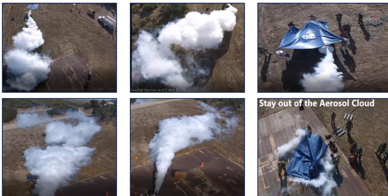
Figure 3-15 Dry Day Releases-double 7/8" Nozzles at 125 psi 68°F and 5 to 8 mph wind
