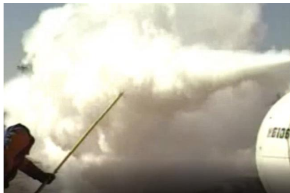
Figure 3-8 Firefighter using a temperature probe to determine the coldest point in the aerosol cloud.
