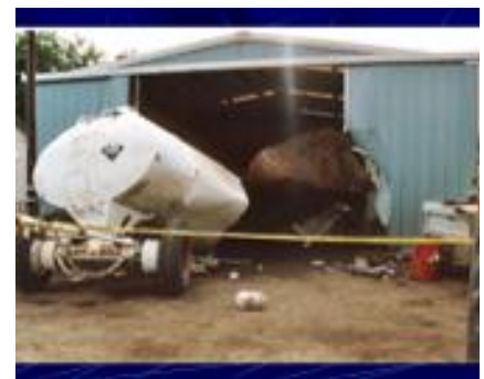
Figure 4-10 Left Trapped liquid blows the liquid line; Right Tank Failure due to Aqueous Mixing with Anhydrous \text{NH}_3
