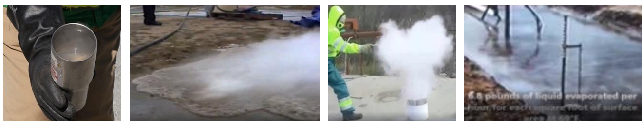
Figure 3-5. Pure \text{NH}_3 2. Ammonia Mixes with Water 3. Aqueous Puff Cloud 4. \text{NH}_3 Liquid Vaporization
