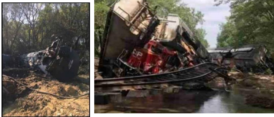
Figure 4-6 The left side picture is the damaged railcar that released the 33,000 gallons of ammonia into the turbulent floodwaters. The Right picture are the railcars and locomotive that landed on the damaged railcar. spread of ammonia vapor impact. Pockets of ammonia entrapped within the mud would occasionally vent from workers and from moving out the railcar debris.
