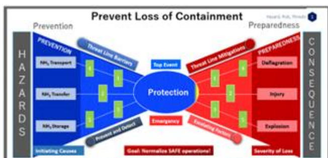
Figure 2-2 ASTI Emergency Response Bowtie Diagram
