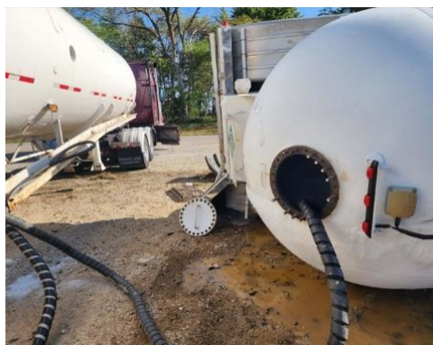
Figure 3-27 Transferring Ammonia Liquid
