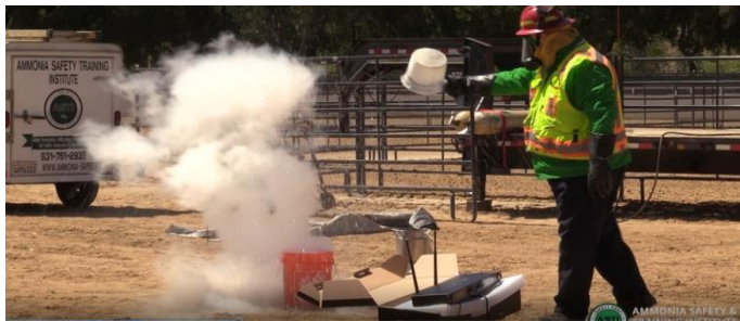
Figure 3-25 Puff Clouds – left picture Water on \text{NH}_3 forms a small aqueous puff cloud.
