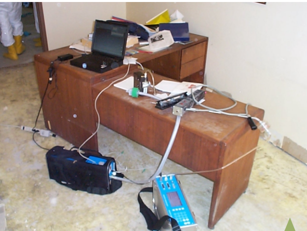
Mercury Monitoring: NIOSH 6009, Lumex and Tracker
