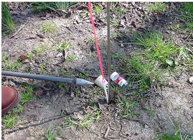
Figure D-3. Installing a passive soil gas module. Courtesy W.L. Gore & Associates, Inc.
